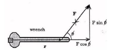
A force **F** is applied to a wrench a displacement **r** from a specific point of rotation (ie. a bolt).
