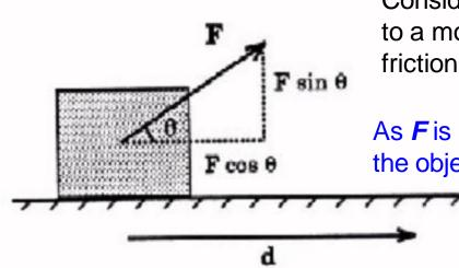
Consider this situation: A force **F** is applied to a moving object as it transverses over a frictionless surface for a displacement, **d**.
