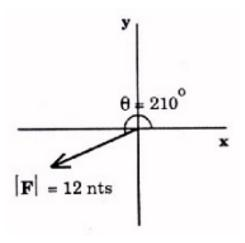
In this picture we have a force vector with magnitude 12 Newtons oriented at 210 degrees with the + x axis. It would be characterized as F = 12 < 210
