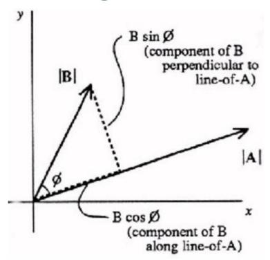
In this figure, vector B has been split into 2 components, one PARALLEL to vector A and one PERPENDICULAR to vector A.
