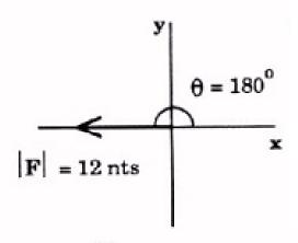
In this picture we have a force vector of 12 Newtons oriented along the -x axis. However, polar notation is relative to the + x axis. Therefore, it would be characterized by F = 12 < 180
