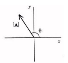
Polar notation defines a vector by designating the vector's magnitude |A| and angle θ relative to the +x axis. Using that notation the vector is written:
